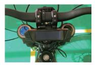
For on-road scenarios, it is recommended to mount the display above the stem to enhance the overall aesthetic of the vehicle. The difference between standard stems and double-clampstems lies in the orientation of the display bracket clamp. The installation results are demonstrated as follows:
