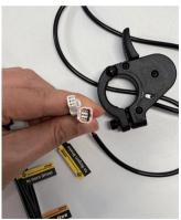
Interface③connects to the electronic brake (thumb brake) harness interface.
