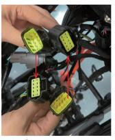
Interface 4 connects to the main bike wiring harness functional interface, with the male connectors connecting to the female connectors respectively.
