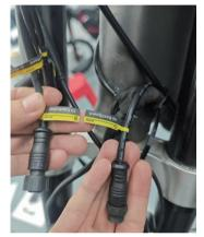
The wire harness connector at the rear of the controller should be as far to the sides as possible, and the upper wire harness should be placed behind the number plate. After the wire harness is tidied up, install the number plate and the side cover. The arrangement effect of the side wire harness is as shown in the figure.
