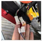
Interface 4 connects to the main vehicle wiring harness interface
