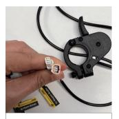
Interface 3 connects to the electronic brake (thumb brake) harness interface.
