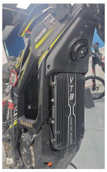
The installed controller should appear as shown in the illustration.
