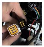
Interface 4 connects to the main vehicle wiring harness interface
