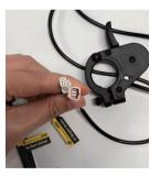
Interface③ connects to the electronic brake (thumb brake) harness interface.
