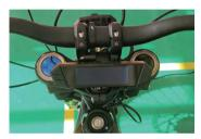
For on-road scenarios, it is recommended to mount the display above the stem to enhance the overall aesthetic of the vehicle. The difference between standard stems and double-clampstems lies in the orientation of the display bracket clamp. The installation results are demonstrated as follows:
