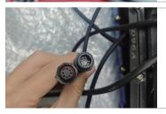
One end of the motor adapter connects to the motor harness interface, while the other end connects to the shorter harness of the controller.
