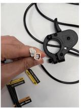
Interface  $\ensuremath{@}$  connects to the regen brake (thumb brake) wiring harness interface.
