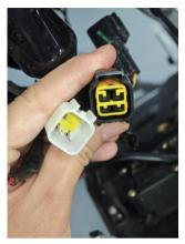
The horn driver connects one end to the main vehicle wiring harness and the other end to the mid-section harness at Interface  $\widehat{\mathbb{ S}}.$
