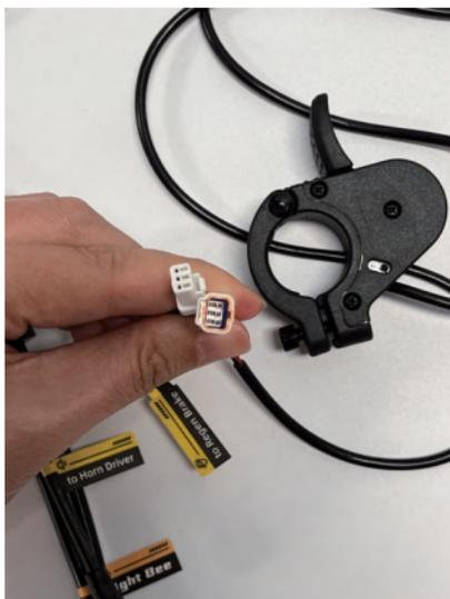
Interface ② connects to the regen brake (thumb brake) wiring harness interface.
