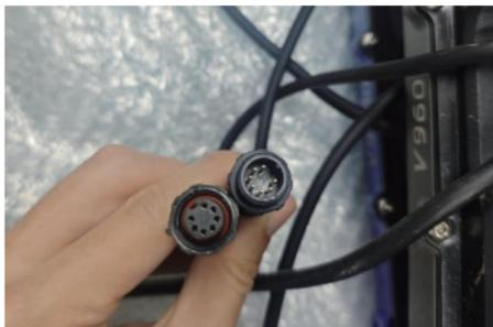
One end of the motor adapter connects to the motor harness interface, while the other end connects to the shorter harness of the controller.
