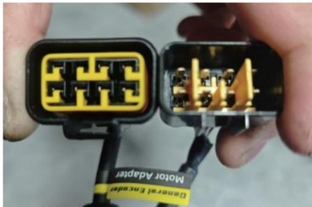
For third-party encoder motors, a general encoder motor adapter is needed.
