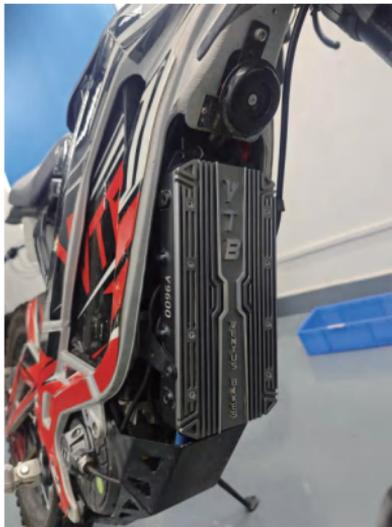
Begin by aligning and securing the lower mounting holes of the controller using screws from the accessory kit, fastening them with a wrench. Adjust the position of the controller to align with the upper mounting holes, then tighten the screws with a wrench. Secure all four mounting screws tightly to ensure the controller is stable and free of movement, and finally, tighten the screws on the top of the motor cover to complete the installation.
