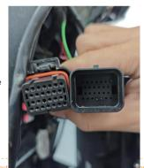
The pins of Interface ① are relatively delicate; exercise caut bending of the pins. When connecting the square plug, a "click" sound indicates that the plug has been securely and correctly connected. If the plug is not fully inserted, it may loosen due to vibrations, resulting in functional abnormalities.
