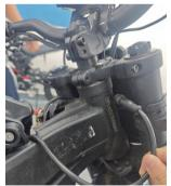
The mid-section wiring harness interface ⑤ should pass through the front of the battery compartment cover and connect to the display at the number plate location. After the wiring harness is organized, install the number plate.
